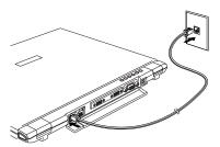
Connecting the internal modem
